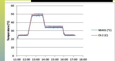
Temperature test result; blue trace: SAW sensor; red trace: thermocouple
